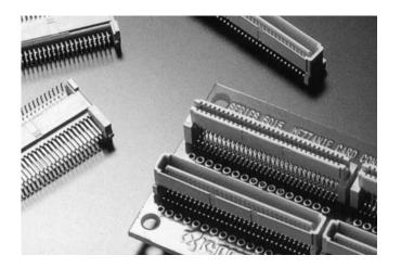
Series 5015 is the board to board connector system that supports the IEEE P-1386 standard for mezzanine card installation in industrial computer applications including VME, Futurebus, and other host boards. At 1.0mm pitch, the 64-position connector can be used with standard PCI and S-Bus mezzanine cards in 64 circuit combinations with mated heights of 8-15mm.
